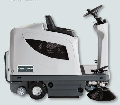
The Terra 4300 sweeper features an aluminum pre-filter panel that traps light bulky debris in the hopper. The pre-filter prevents clogging while offering optimum dust control. And its electric filter shaker provides excellent filter clean-back. The large four-sided steel manual dump debris hopper allows for maximum debris capacity without overflow. The hopper is easy to remove, while the dolly wheels provide a quick method to transport and empty dirt and large debris.
