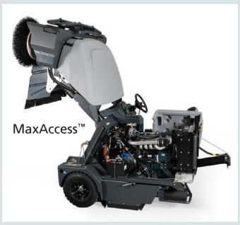
MaxAccess<sup>™</sup> interlocking compartments allow for industrybest accessibility of critical components to expedite service and repair.
