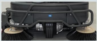
Don't let the smooth, precise acceleration of its maintenance-free AC brushless propulsion drive fool you. With an industrial bumper, frame-mounted deflectors and a tubular, steel construction all specifically engineered for the most severe industrial applications, the SC6500 is as tough as they come and built to last.
