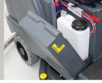
Removable, high capacity detergent cartridge for sustained flexible cleaning is available with optional EcoFlex<sup>™</sup> System.
