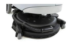
The SC351's rotating deck allows for both forward and backward scrubbing. Operators can push the machine forward in all directions like a "normal" scrubber. But, if the application requires, operators can quickly flip the machine up, triggering the deck to rotate completely for backward scrubbing performance. The scrub deck efficiently guides the wheels for superior edge cleaning.
