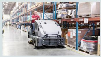
SmartFlow<sup>™</sup> adjusts solution flow with the machine's speed, using water and chemicals. Proportionally higher productivity with fewer dump and refill cycles per tankful
