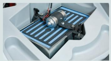
High-capacity Donaldson PowerCore® UltraWeb® nanofilter synthetic media filter with MERV 13 rating with a variable-frequency shaker. Provides superior dust/dirt holding capacity in a more compact package for longer filter life and improved dust control compared to conventional pleated filters
